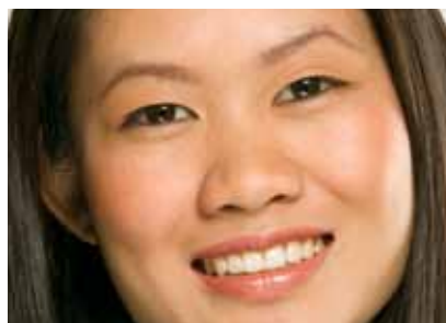
A 5% tone shift during plating at the 50% mid-tone (-5% M) and loss of 1 & 2 % highlight dots.
